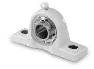
Housing Material is a Reinforced PBT (Polybutylene Terephthalate) that provides extreme low water absorption, and exceptional dimensional stability. With excellent resistance to chemical attack and high environmental stress crack resistance, these units provide excellent wear properties. Housings are supplied with seamless stainless bushings and zerk fitting.
