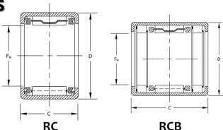
The design calls for caged construction that includes an interior spring that wedges against the needle rollers and allows free running in one direction but locks the clutch with the shaft when rotated in the opposite direction. The bearings are easily installed with a press fit in the housing.
