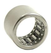
BL Drawn Cup Roller Clutch bearings are designed to transmit torque between the shaft & housing in one direction while allowing free overrun in the opposite direction. These are ideal for applications where one-directional movement is needed with backstopping or indexing capabilities such as: conveyor rollers, rack indexing drives, timing motors, paper feed rolls, and motor backstops
